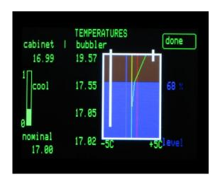
The bubbler condition monitor shows the fill level and the temperatures inside the bubbler.
